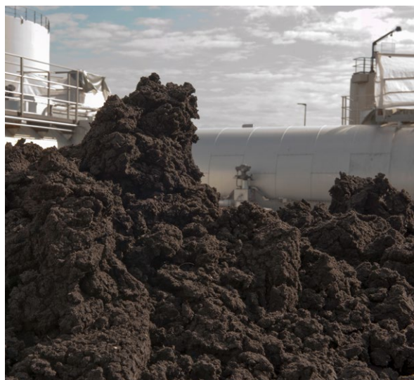
Dewatered sewage sludge
